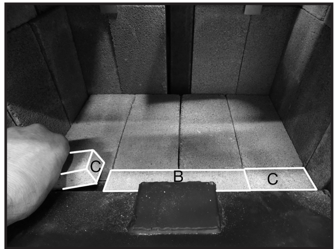
Figure 19: Narrow front bricks in place.
